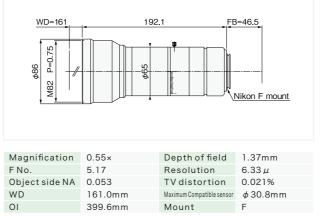
\* Indicated specifications are design values. \* Resolution indicates a theoretical resolution at a wavelength of 550nm. \*Depth of field is calculating assuming a horizontal 320 TV resolution using 1/2 inch camera (permissible circle of confusion 40 µ).
