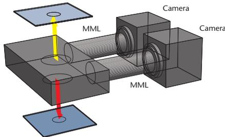
A space-saving optical system for attaching 2 opposite-facing objects with accuracy.
