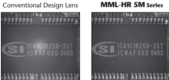
Please note that although the lens is structured to suppress hot spots, hot spots will occur for mat surface work.
