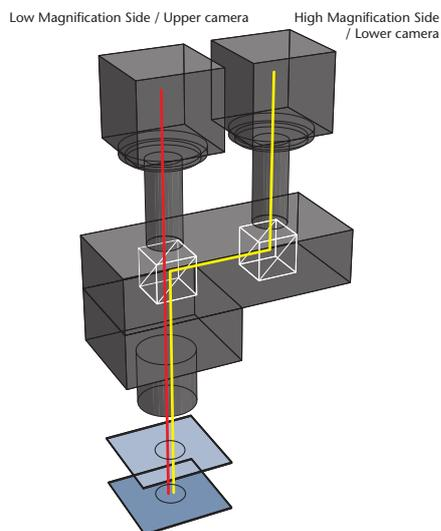
A space-saving optical system that is used to simultaneously observe an object at two focus distances, and two magnifications on one optical path utilizing a specific prism structure.
