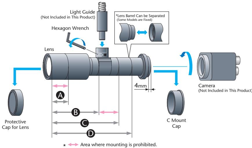
\*1 Where the lens tube segment in the table is marked with an "x", the lens cannot be detached at that point.
