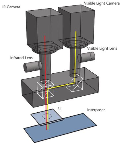
A complete lens and lighting system which uses infrared rays to transmit through a Si, GaAs, or Ge substrate to recognize IR penetration patterns.
