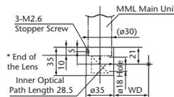
\*WD in the diagrams is the lens working distance minus the inner optical path length.
