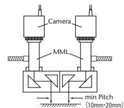
\*WD in the diagrams is the lens working distance minus the inner optical path length.
