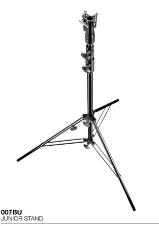
Such family is the "intermediate" in Manfrotto light stands range. Heights covered from 124cm/48.8in to 477cm/187.8in. Payload supported go from 12kg/26.4lb to 40kg/88.2lb. Components are all in aluminum.
